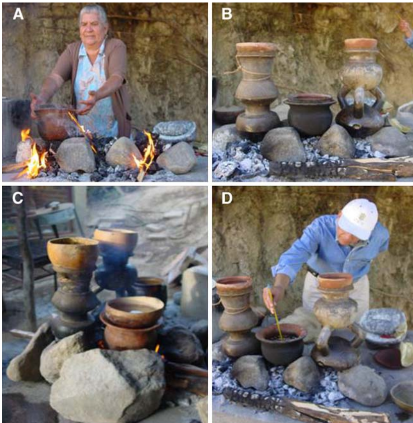
Fig. 4. Simulation of ancient distillation method using the trifid and gourd-shaped experimental stills. (A) Building a stone firepit using burning wood. (B) Using ceramic accessories. (C) Using gourd ( L. siceraria ) accessories. (D) Scoring of temperatures in the bean pot as a reference.
